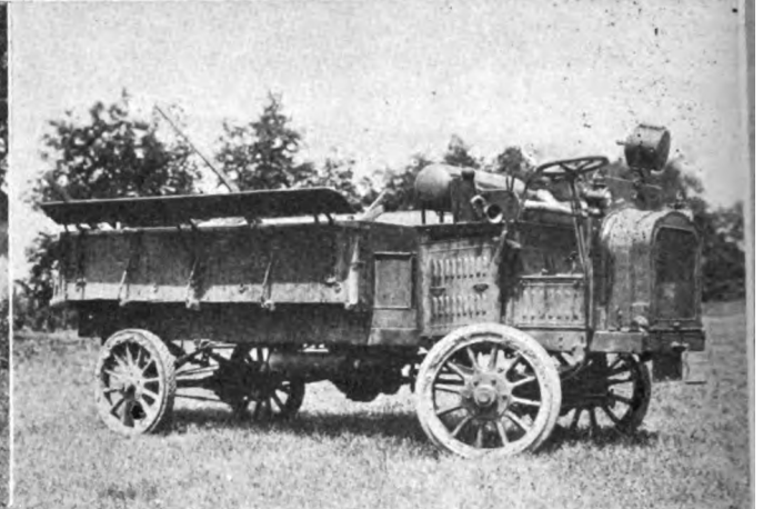
Flareboard bodies on 1½-ton chassis are most popular for a around army use
